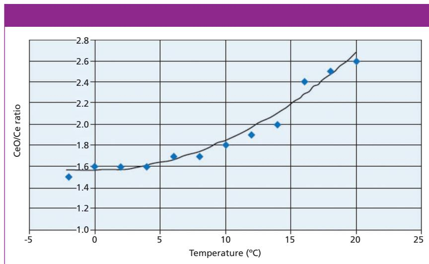
**Figure 4:** Improvement in oxide ratio performance (CeO/Ce) using a chilled spray chamber.
