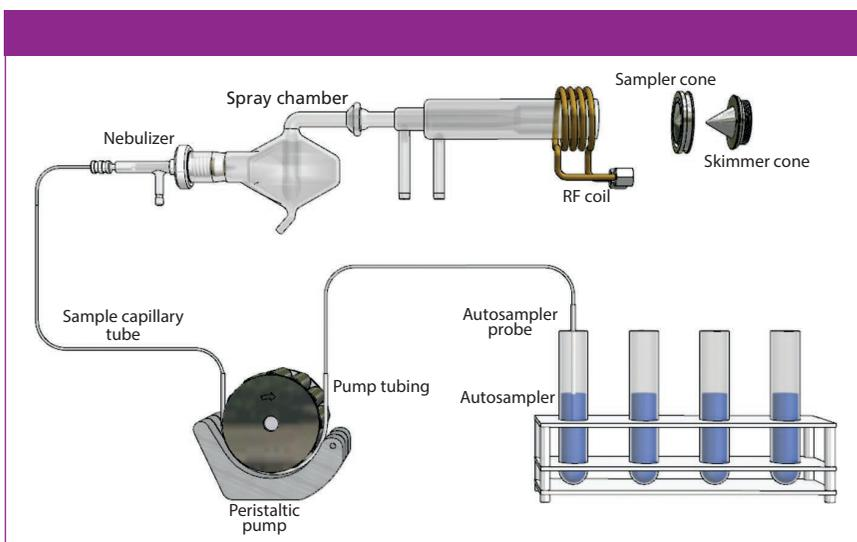
**Figure 2:** A close-up of the ICP-MS sample introduction area.
