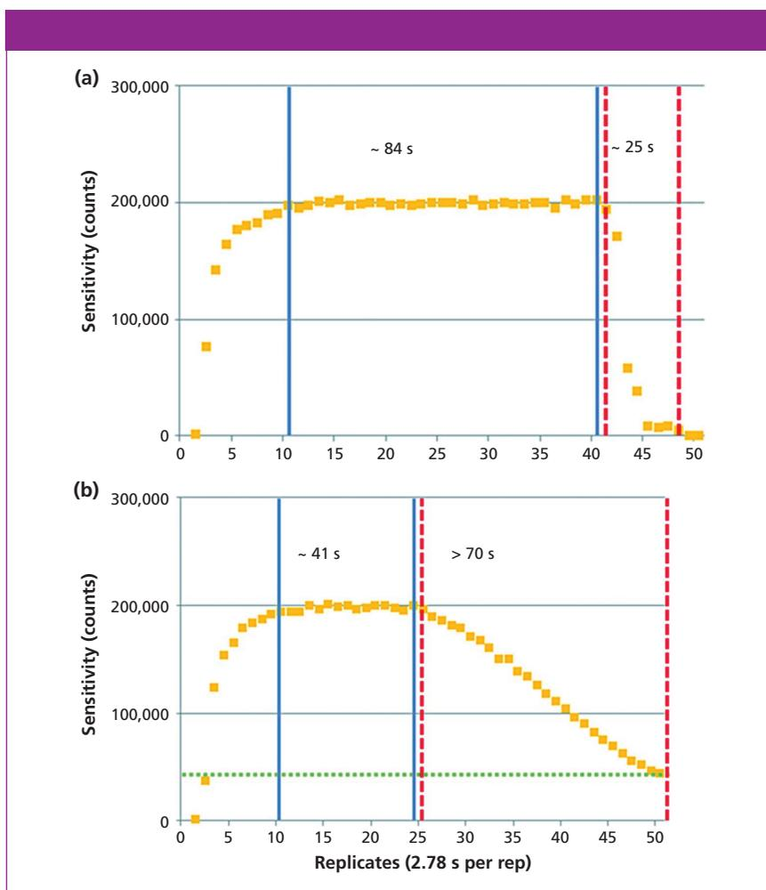
**Figure 6:** Results from injections with a bubble injector (a) on and (b) off. The use of a bubble injector and optimum positioning of the autosampler probe enable a twofold increase in available measurement time and greater than a threefold decrease in washout time.
