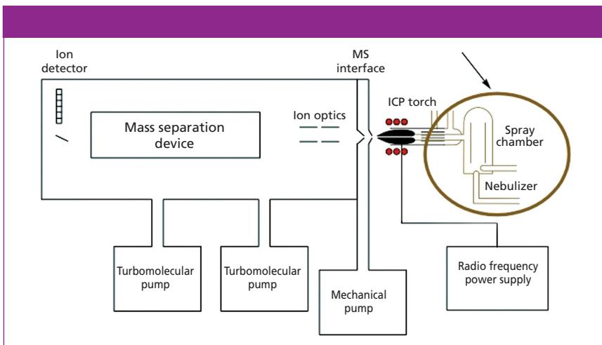
**Figure 1:** Major instrumental components of an ICP-MS system.
