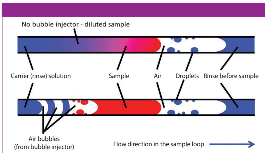
**Figure 5:** The principle of injecting air bubbles at the end of the sample plug.
